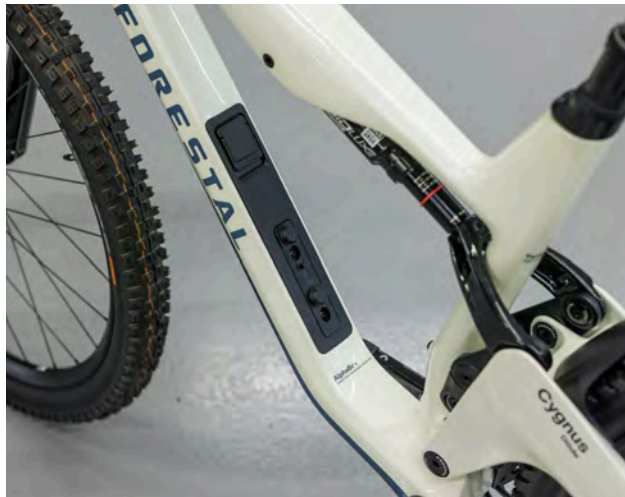
Internal storage lid with integrated magnetic closure and bottle base
